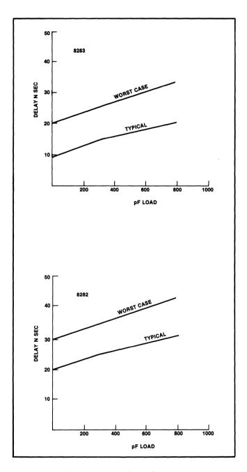
Figure 6. Output Delay vs. Capacitance
